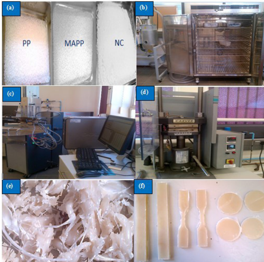
Figure 3: Image of methodology processes: (a) raw materials, (b) oven dryer, (c) rheomixer, (d) compression mold, (e) premixed sample, and (f) molded-shaped samples
